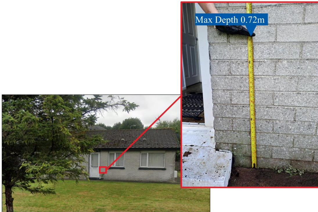
Figure 58: Estimated Depth of Flooding at the Residential Property Opposite Chadwick's
