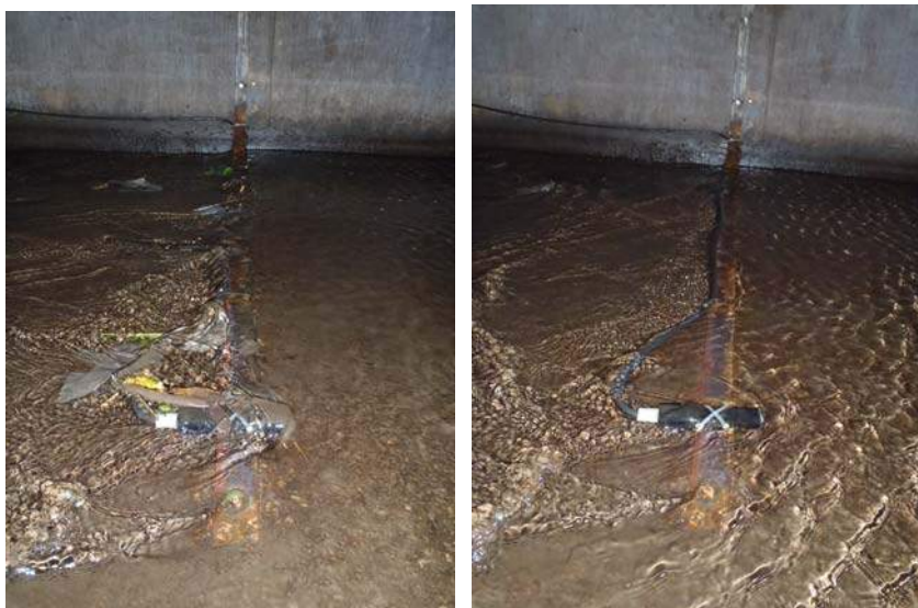
Fig 47: FM3 AV Probe before and after cleaning during low water levels
