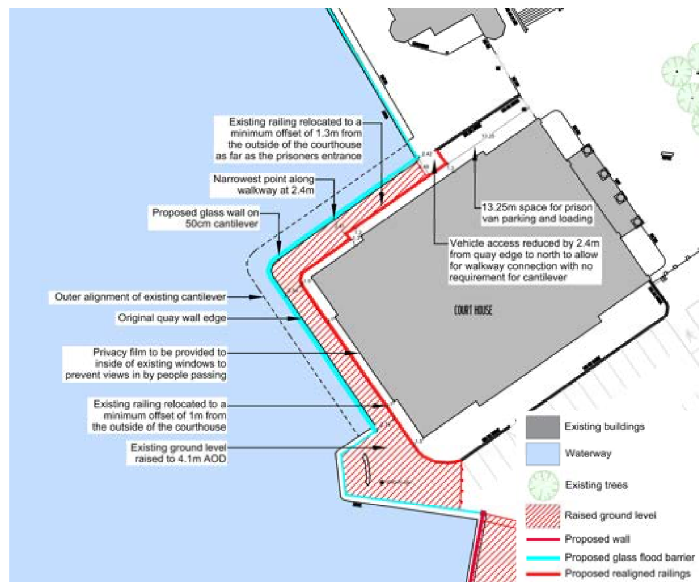
Alternative Option 3: Courthouse railings realigned, 50cm cantilever and 13.25m prison van area.
