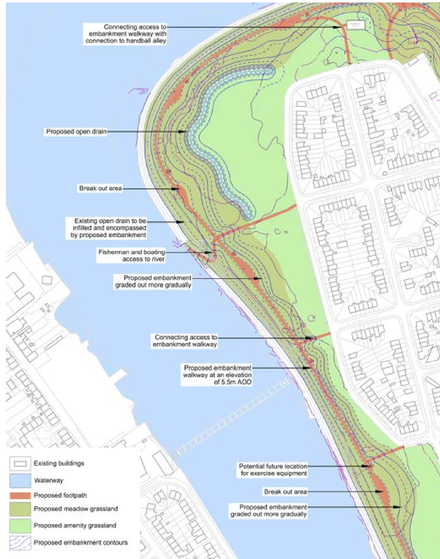
Plan illustrating extent of the proposed northwest embankment and the replacement open drain
