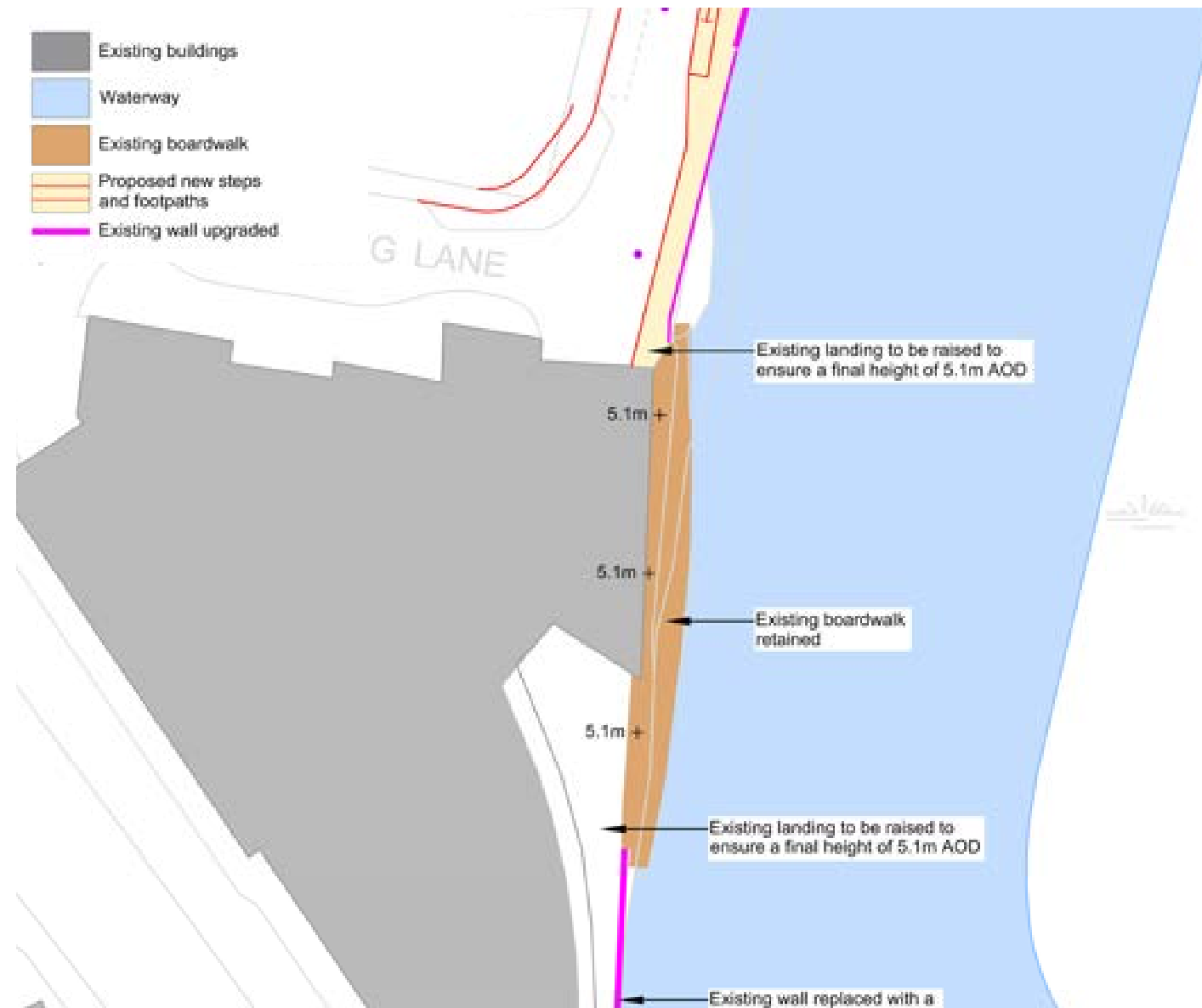
Plan illustrating the extent of the boardwalk and the two landings to be raised.
