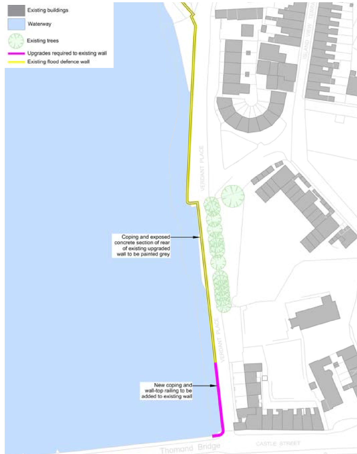
Extent of wall to be upgraded with replacement railing.
