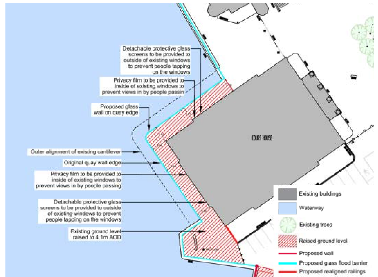
Alternative Option 2: Cantilever and Courthouse railing removed.
