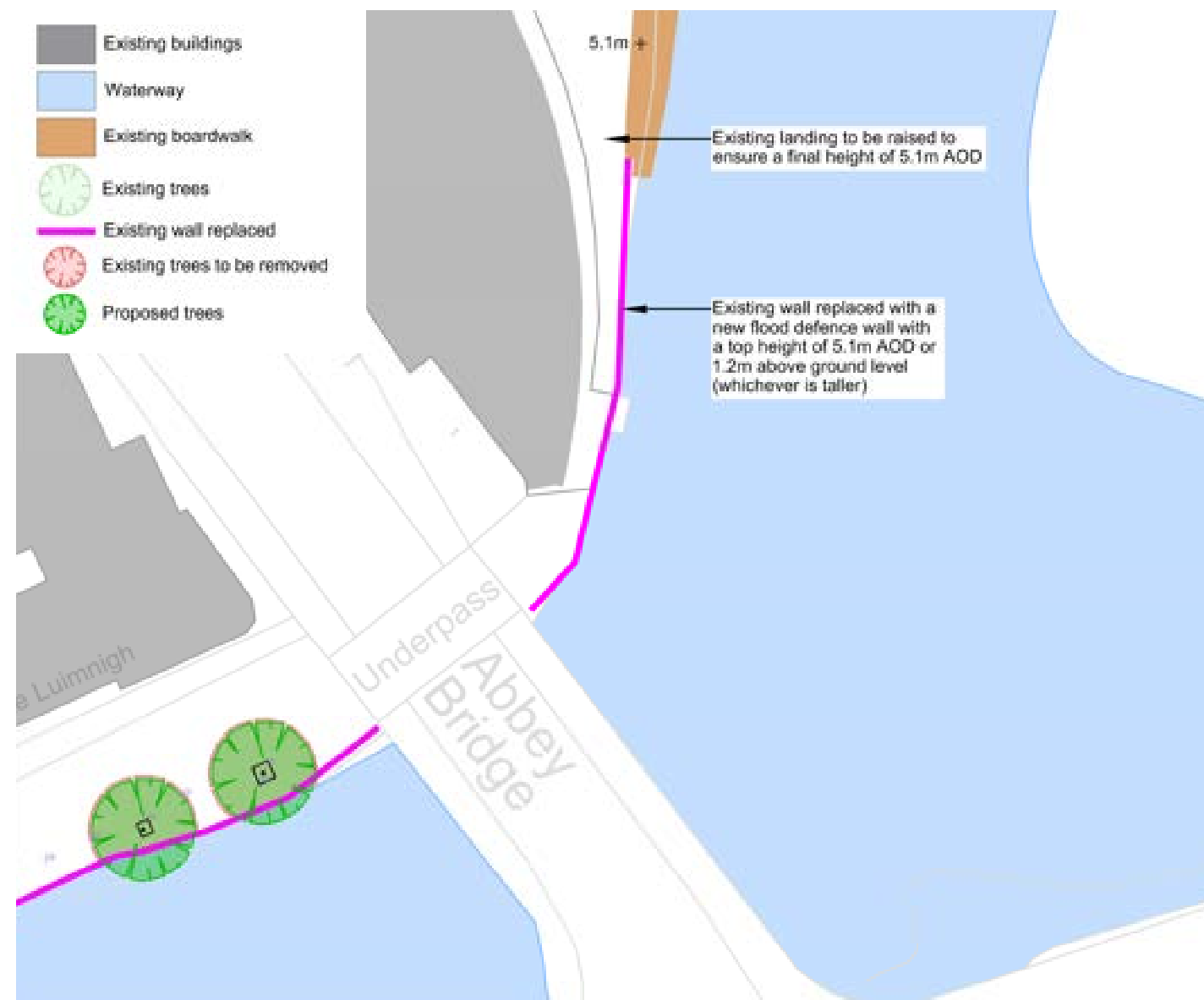
Plan illustrating the extent of wall to be upgraded between the boardwalk and Abbey Bridge.
