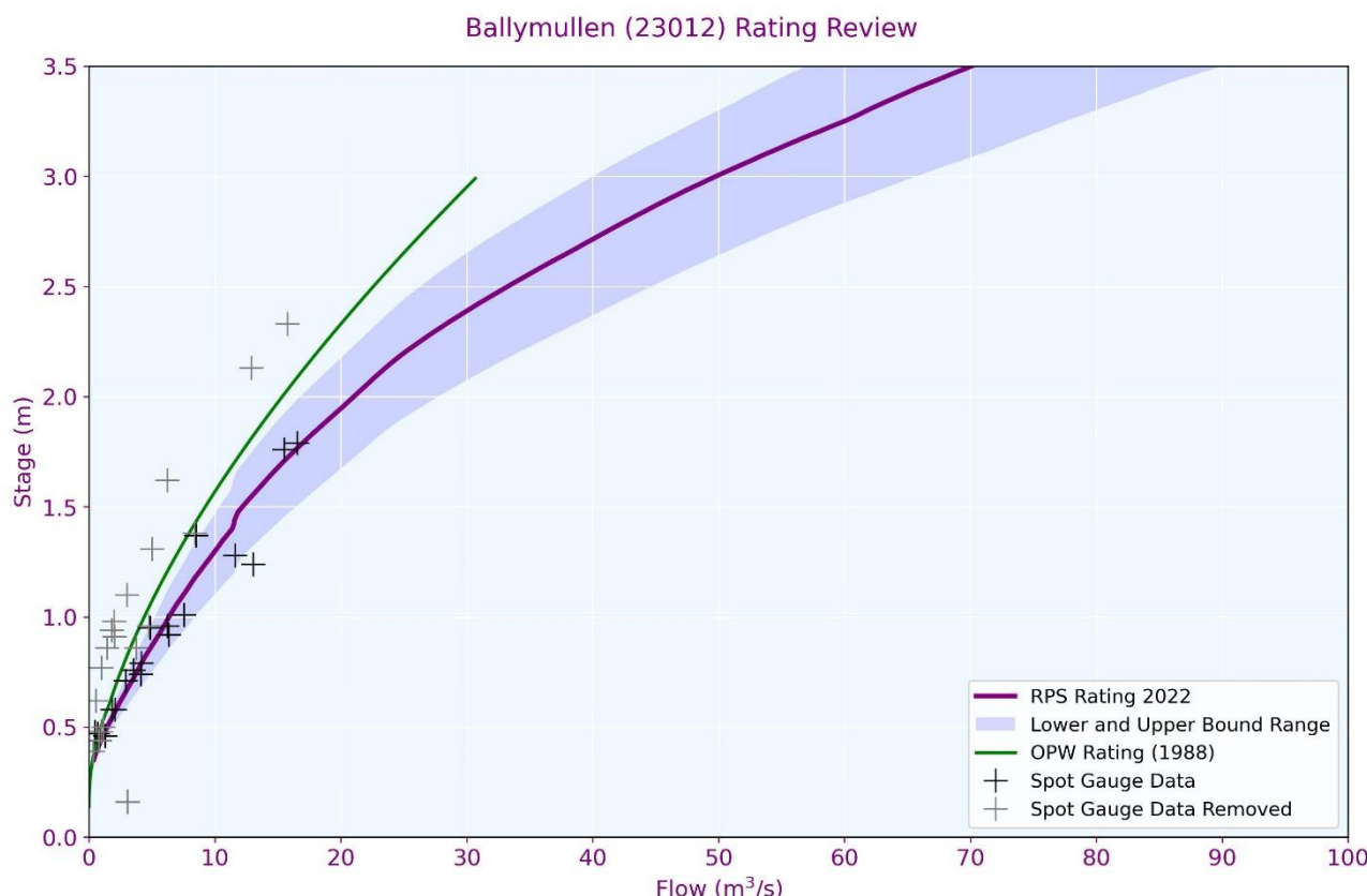
Figure 2.10: OPW Rating (1988) Compared to RPS Proposed Rating (2022) which shows a clear shift to a less steep rating curve which results in higher flows. Also included is the spot gaugings and those which were removed for the development of RPS proposed Rating (2022)
