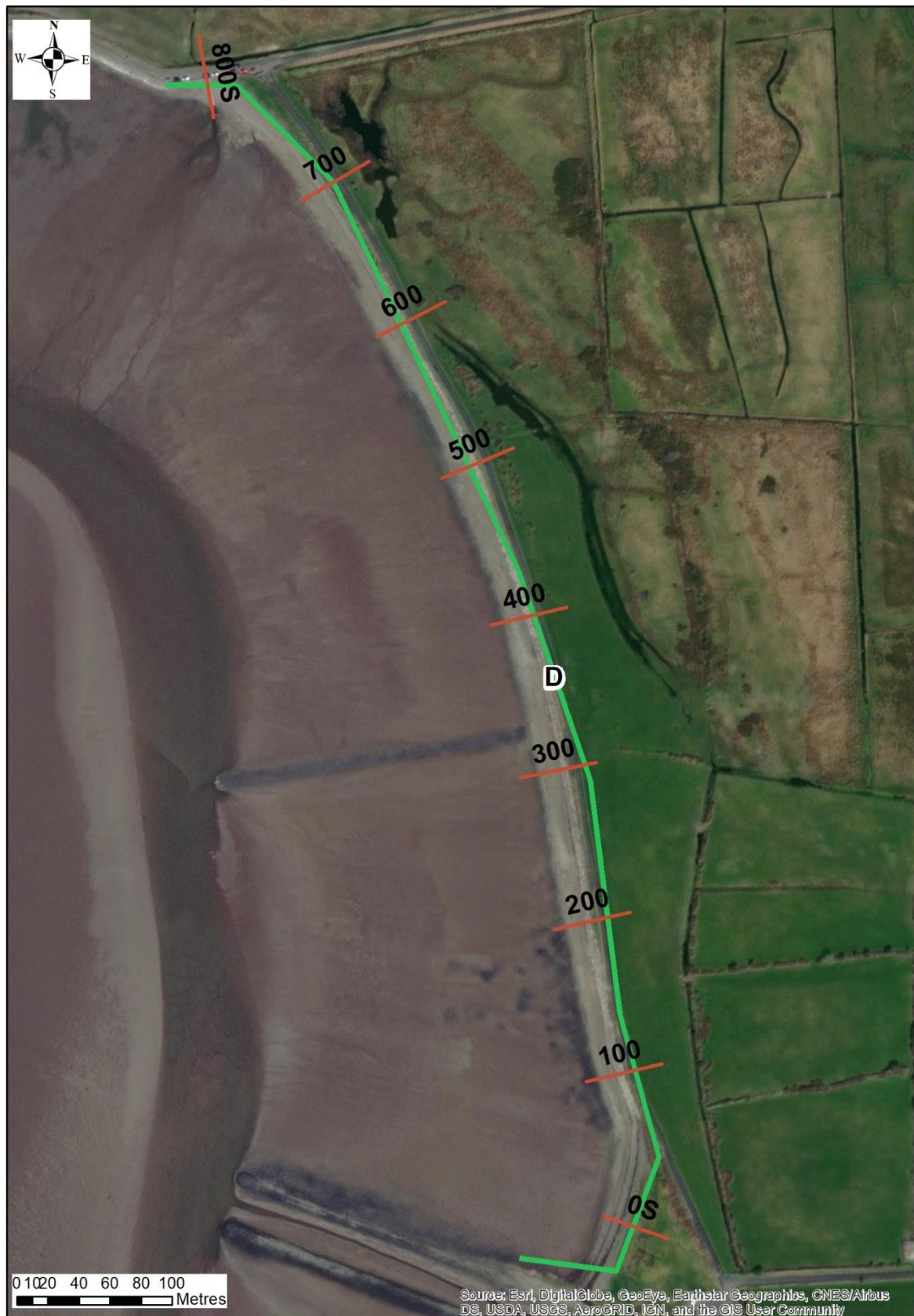
Figure 6.11: Cross Sections Assessed at CAPO D
