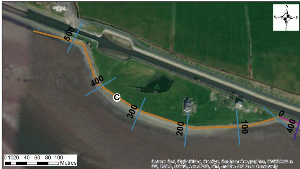
Figure 6.9: Cross Sections Assessed at CAPO C
