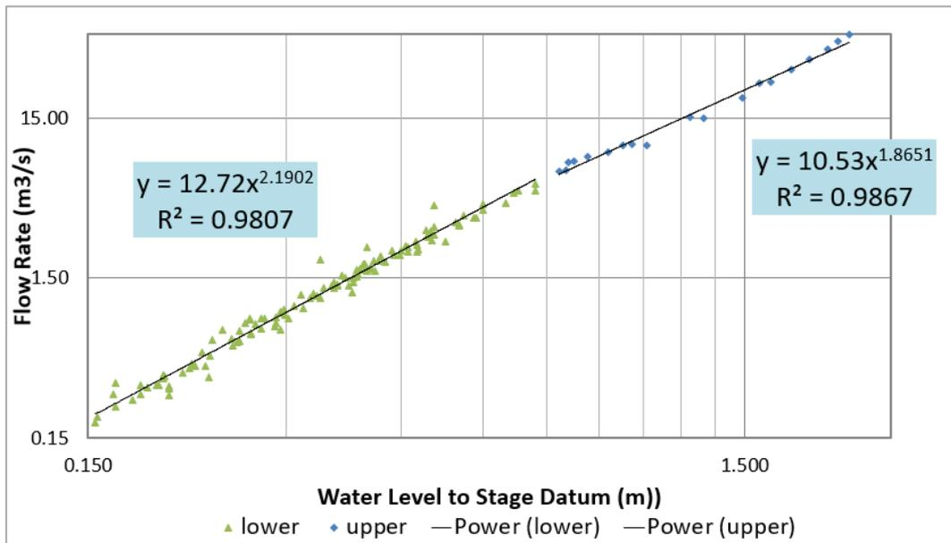
**Figure 5-13: Revised Curve Fitting After Correcting the Datum Value of Spot Gauging**
