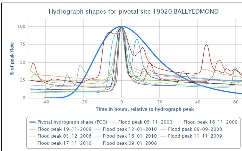
Figure 8-1: Design Flow Hydrograph Shape
