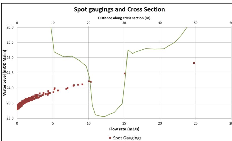
Figure 5-5: Spot Gauging and Cross Section
