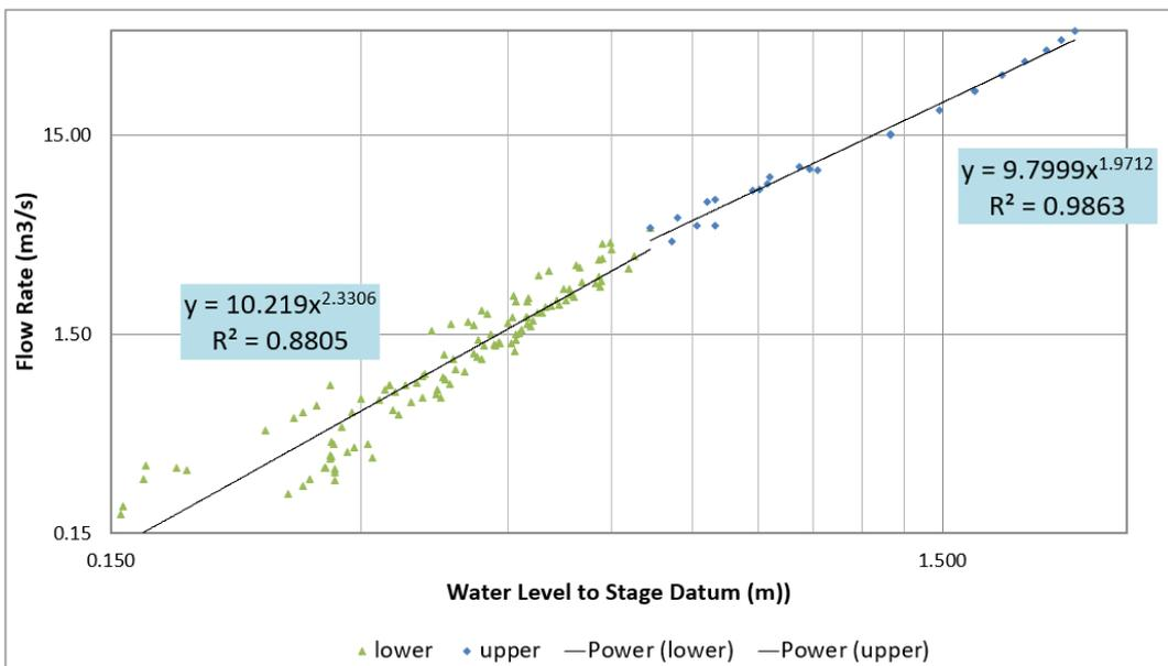
**Figure 5-11: Fitting Rating Curve**
