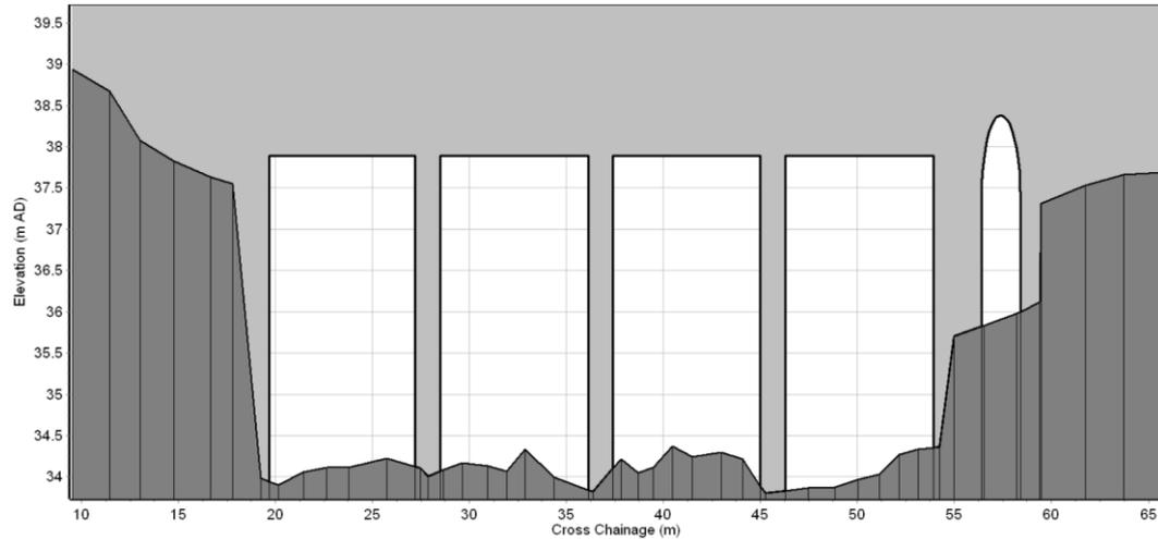
**Figure 26: Configuration of East Bridge's sluice gates currently in place**
