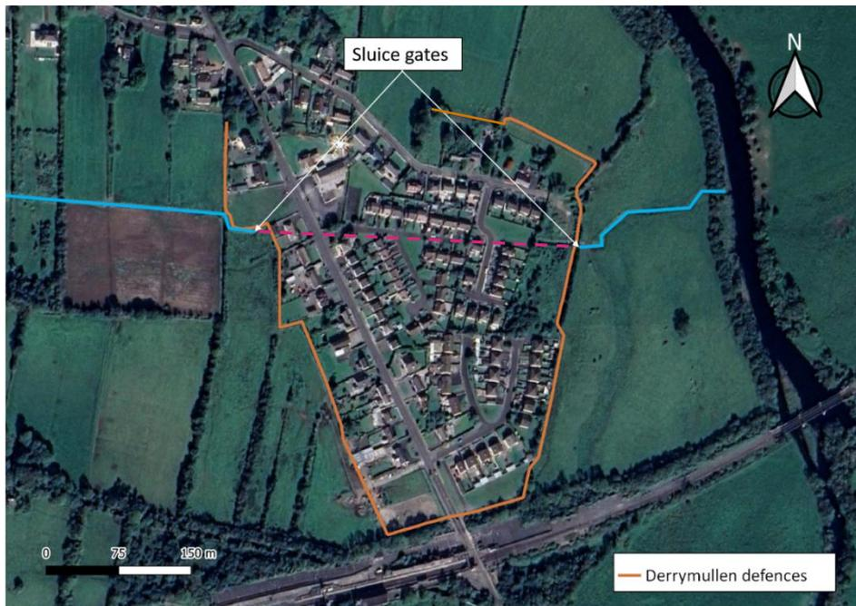
**Figure 30: Simplified schematic of the Derrymullen Flood defence scheme**
