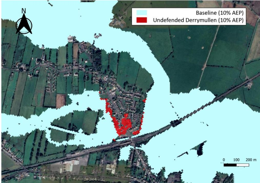
**Figure 57: Comparison of flood extents for the Derrymullen Undefended scenario (10% AEP)**
