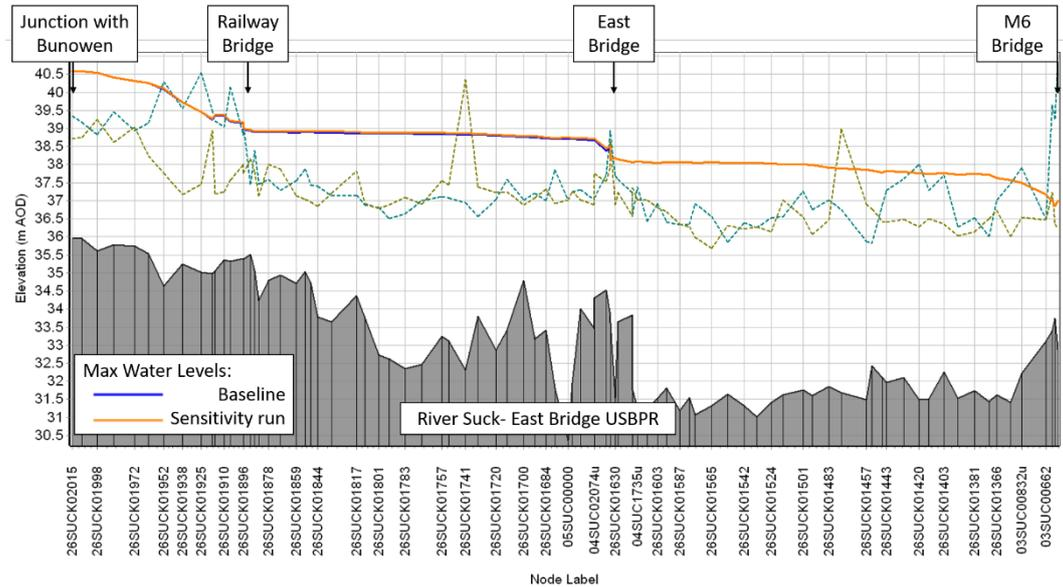
**Figure 54: Longitudinal plot of the Max WLs along the River Suck - baseline Q100 model with East Bridge defined as a USBPR**
