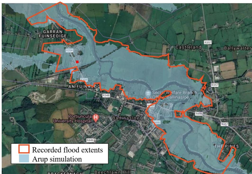
**Figure 41: Comparison between the recorded flood extents and Arup's simulation result.**
