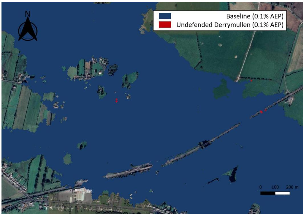
**Figure 59: Comparison of flood extents for the Derrymullen Undefended scenario (0.1% AEP)**
