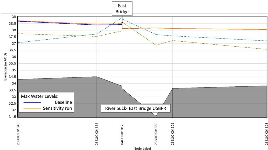
**Figure 55: Zoomed in longitudinal plot of the Max WLs along the River Suck - baseline Q100 model with East Bridge defined as a USBPR**
