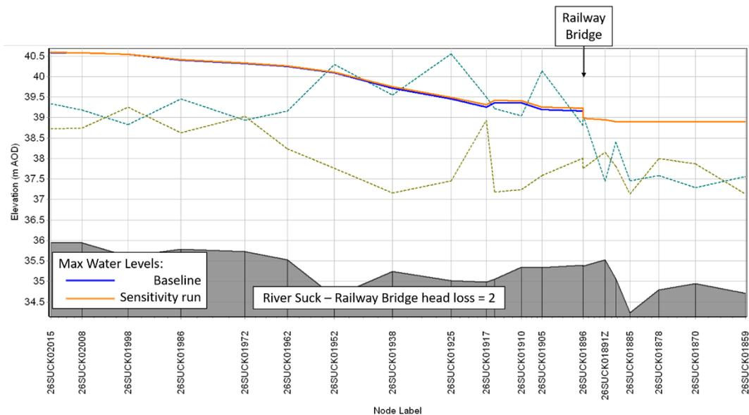
**Figure 53: Zoomed in longitudinal plot of the Max WLs along the River Suck - baseline Q100 model with Railway Bridge head-loss coefficient sensitivity analysis**
