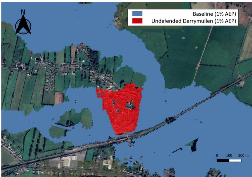
**Figure 58: Comparison of flood extents for the Derrymullen Undefended scenario (1% AEP)**
