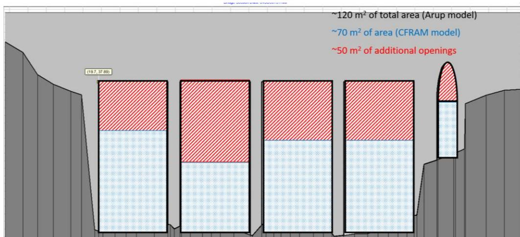
**Figure 27: Comparison of East Bridge sluice gates configurations**
