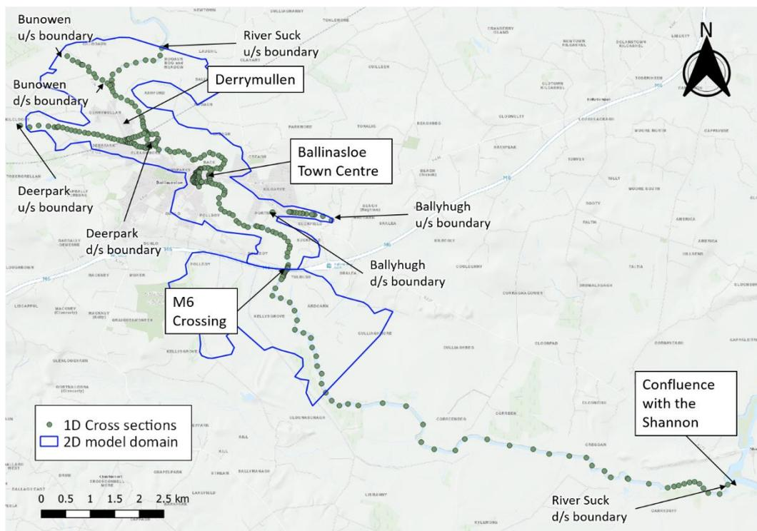
**Figure 20: Ballinasloe FRS model - 2D model domain (blue polyline) and 1D model cross sections (green nodes)**
