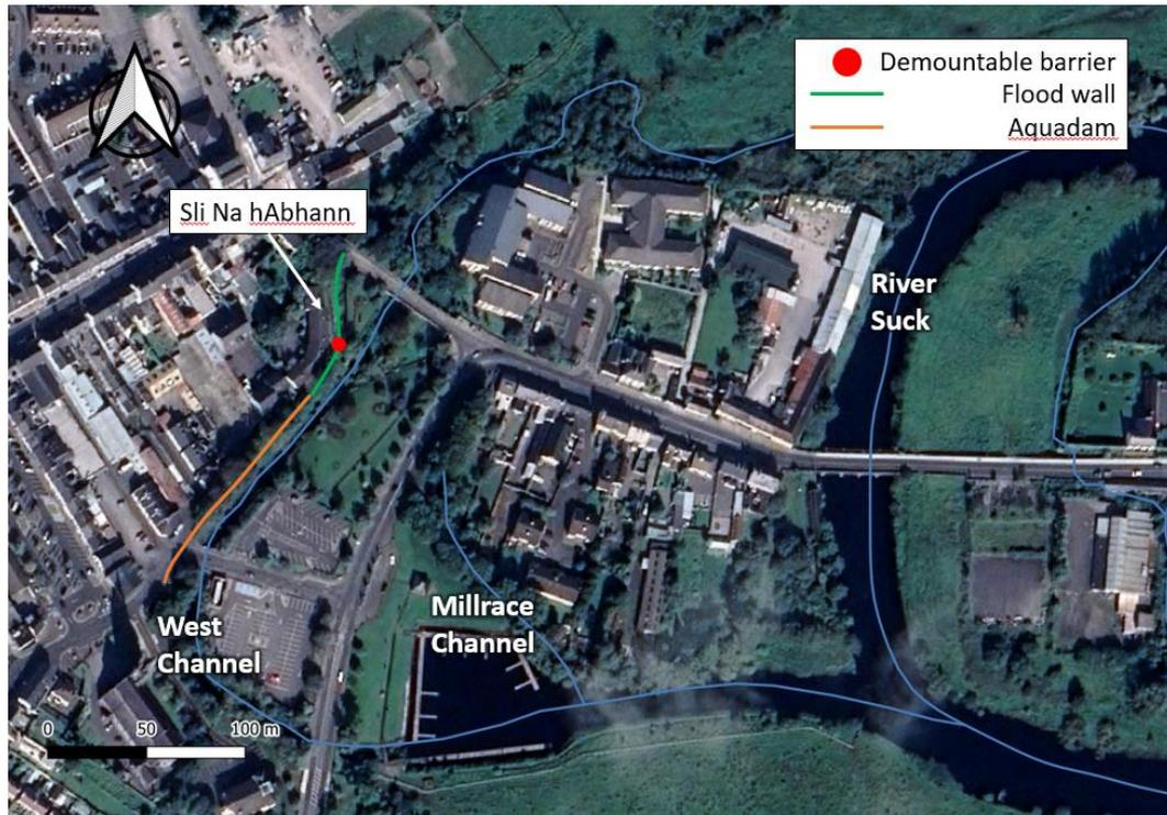
**Figure 32: Indicative alignment of temporary flood defence measures**
