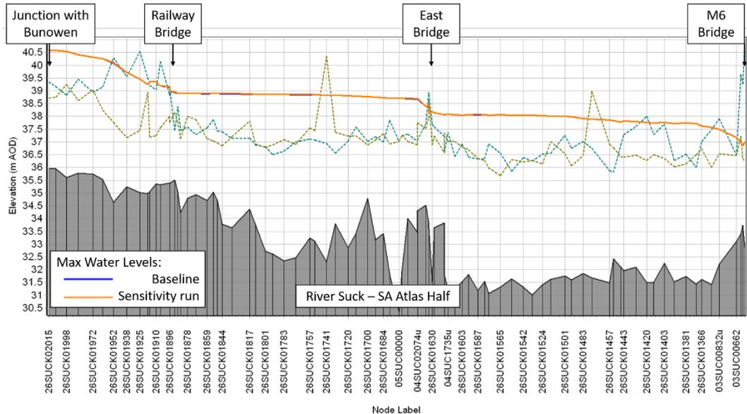
**Figure 56: Longitudinal plot of the Max WLs along the River Suck - baseline Q100 model with Atlas channels sensitivity run**
