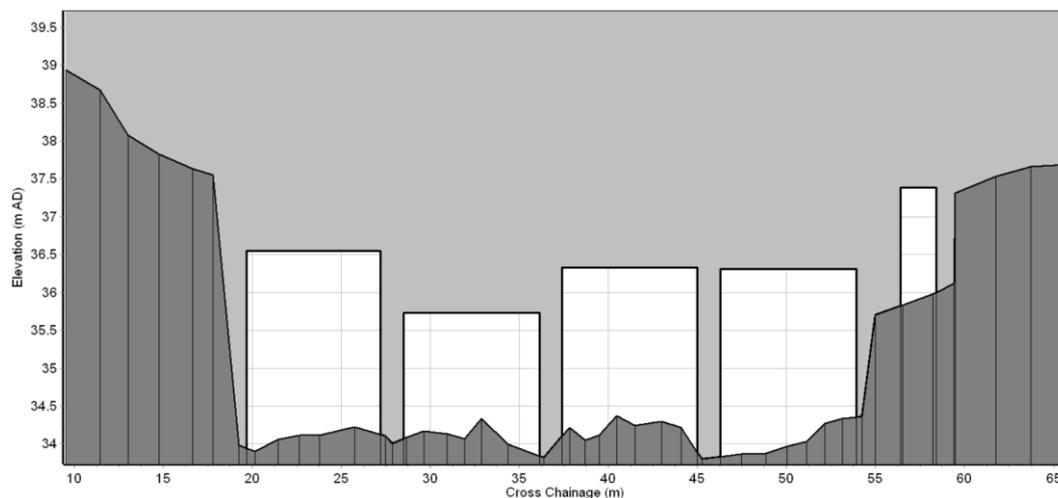
**Figure 25: Configuration of East Bridge's sluice gates up to 2012**
