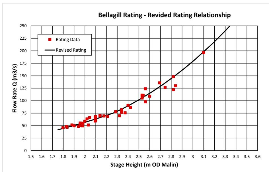
**Figure 17: Revised rating curve for Bellagill**
