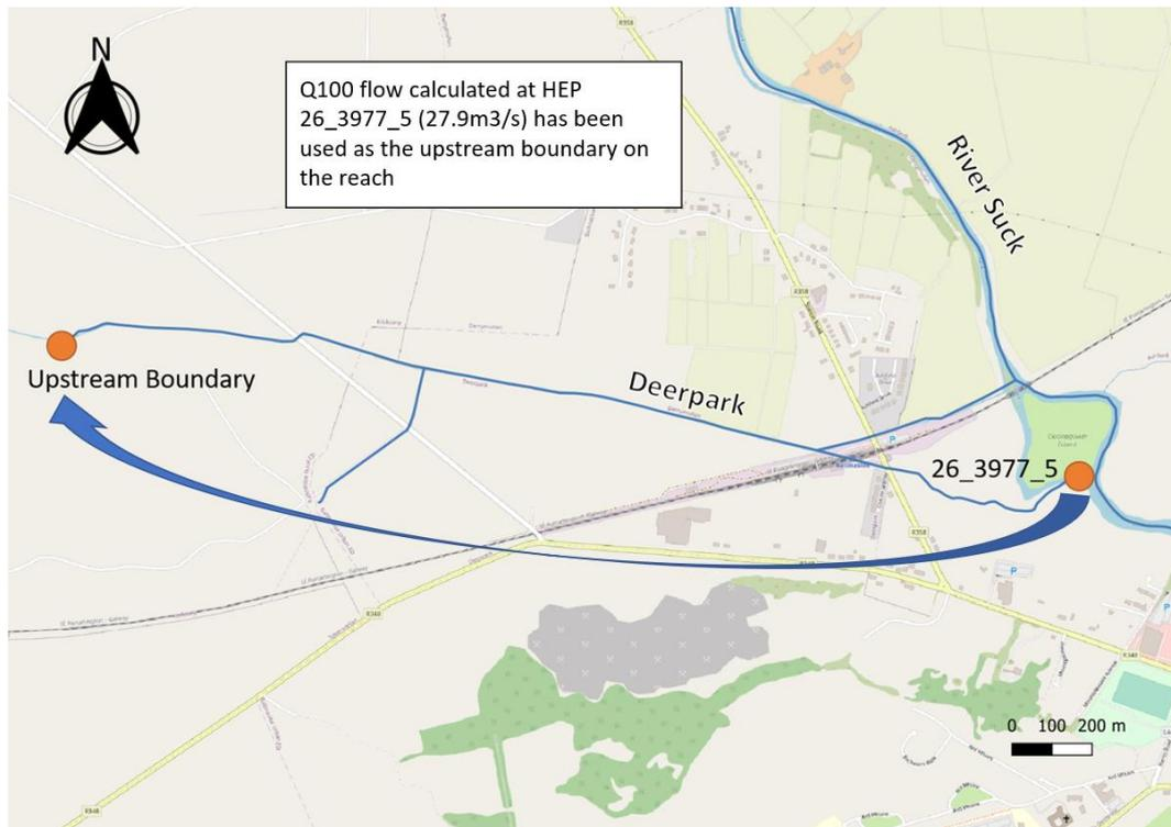
**Figure 19: Setting the flow on the Deerpark Stream**
