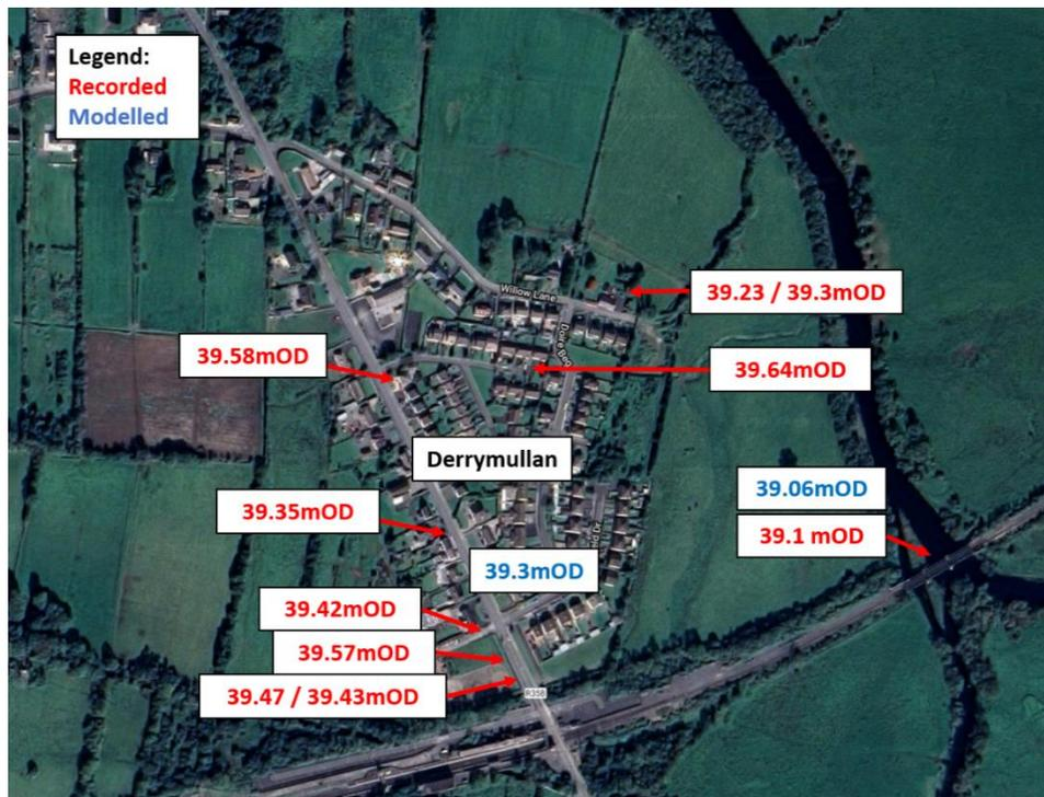
**Figure 42: Maximum water levels at Derrymullen**
