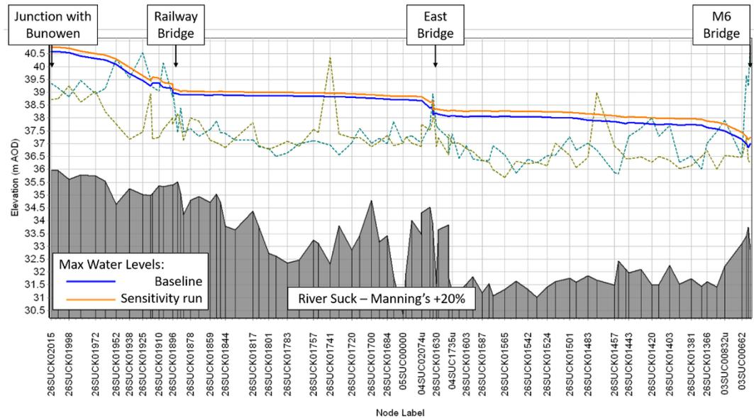
**Figure 47: Longitudinal plot of the Maximum WLS along the River Suck - baseline Q100 model with 20% increase in Manning's n**
