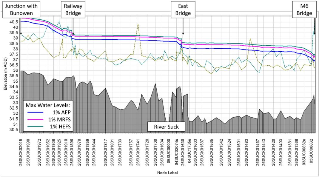
**Figure 60: Longitudinal plot for the Q100 Climate Change runs**
