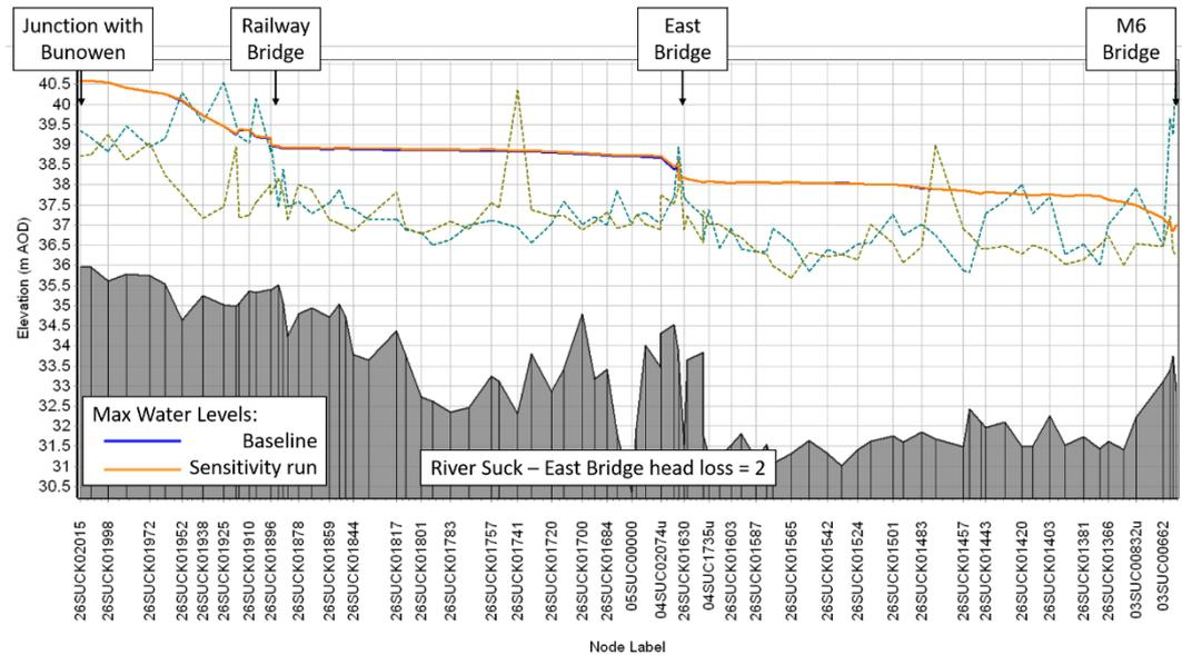
**Figure 50: Longitudinal plot of the Max WLs along the River Suck - baseline Q100 model with East Bridge head-loss coefficient sensitivity analysis**
