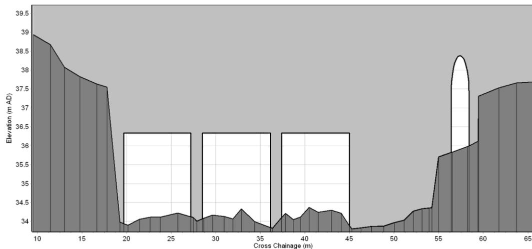
**Figure 23: Configuration of the East Bridge's sluice gates during the 2009 event**
