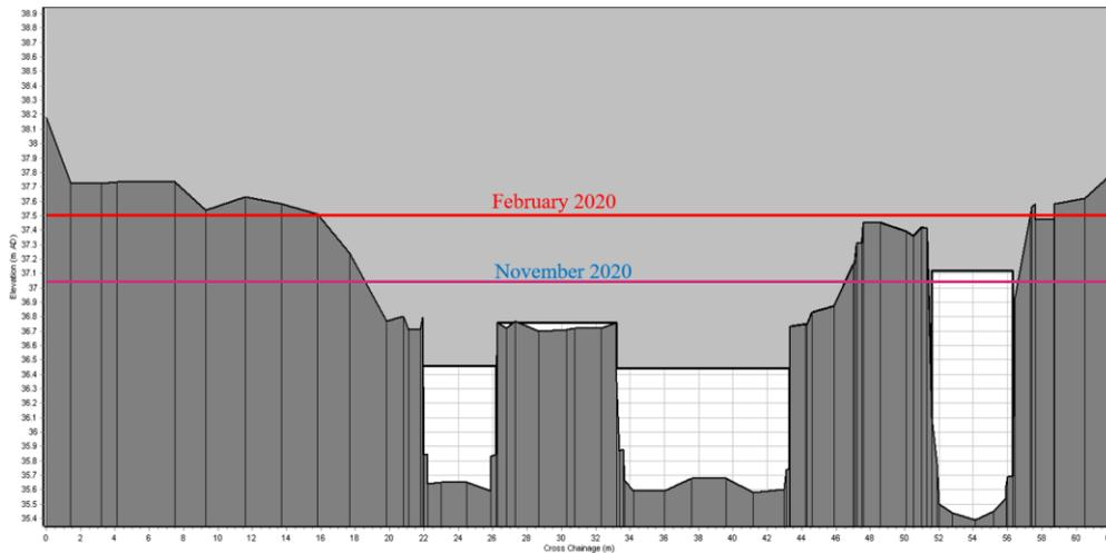
**Figure 39: Pedestrian bridge geometry with maximum water levels for both 2020 events superimposed**
