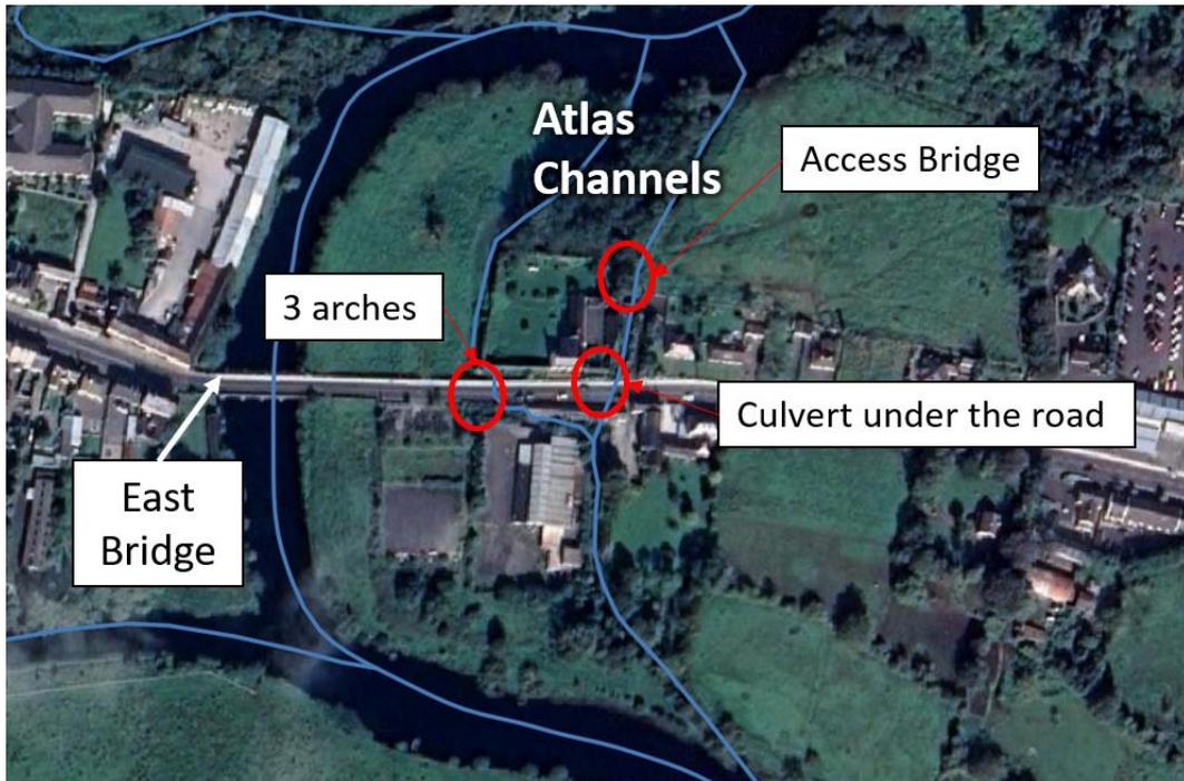
**Figure 28: Atlas channels and modelled structures**
