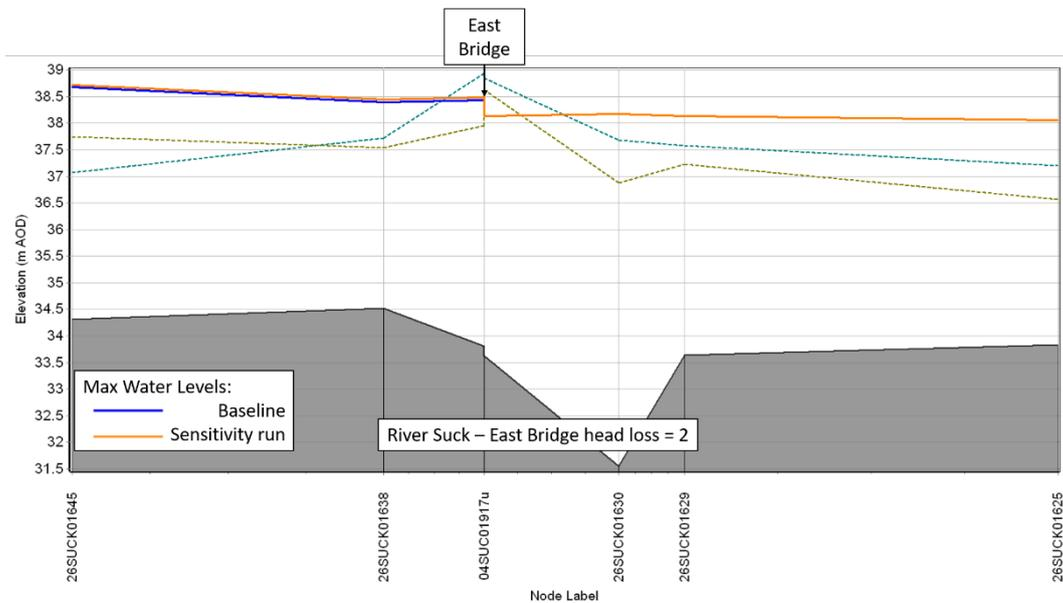
**Figure 51: Zoomed in longitudinal plot of the Max WLs along the River Suck - baseline Q100 model with East Bridge head-loss coefficient sensitivity analysis**
