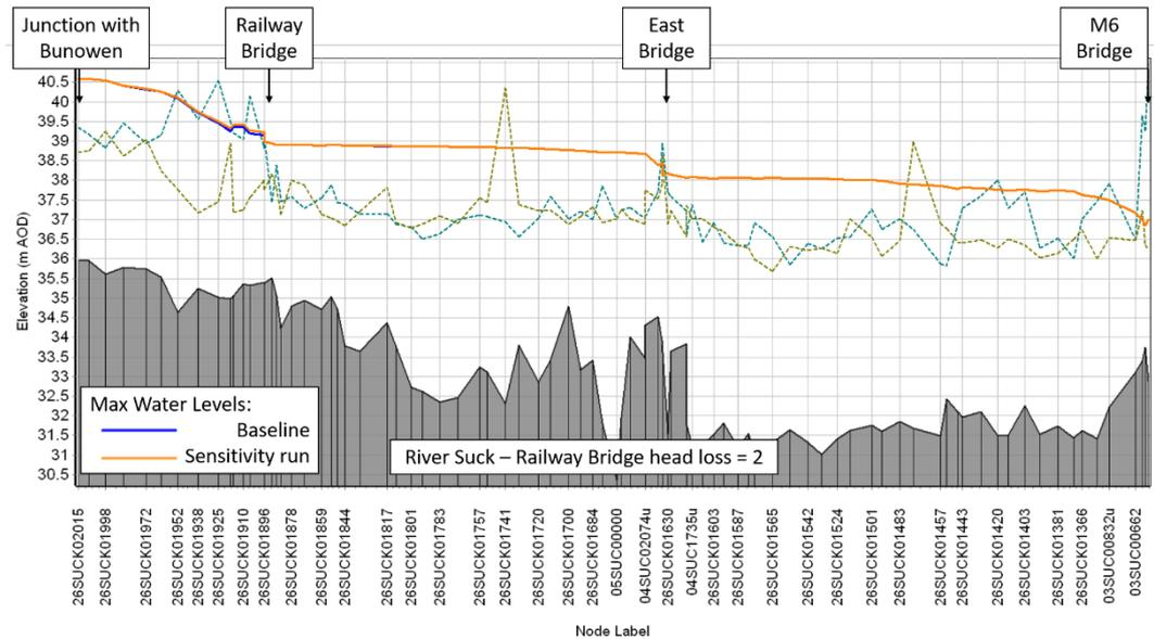
**Figure 52: Longitudinal plot of the Max WLs along the River Suck - baseline Q100 model with Railway Bridge head-loss coefficient sensitivity analysis**
