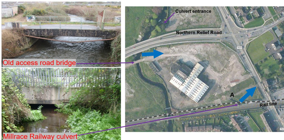
Figure 5.16 Mechanisms of flooding North of the Railway Line
