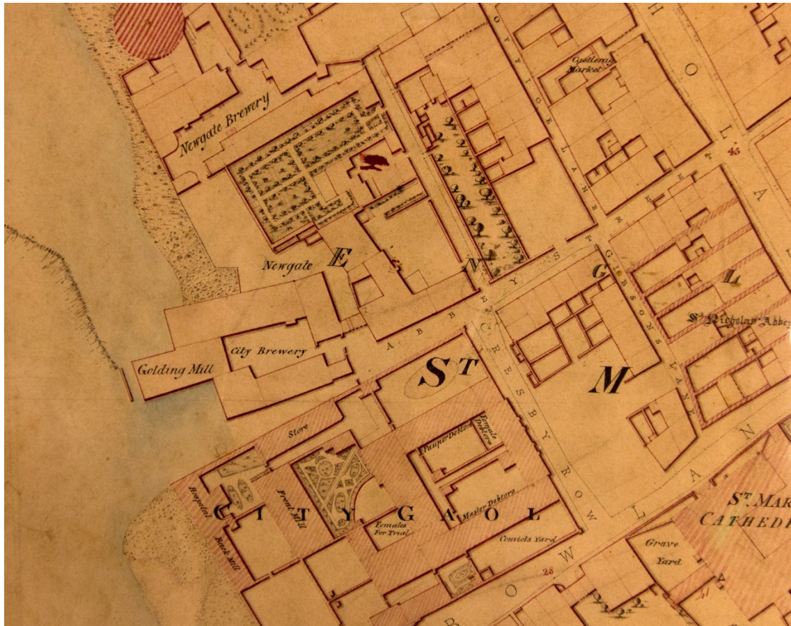
Figure 13 Extract from OS map 1840, note linear feature in front of mill, this may have supported the mill wheel.
