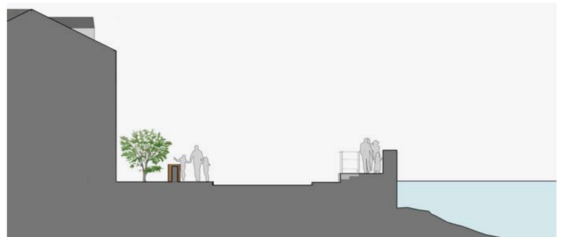
Illustrative section through Sir Harry's Mall and the proposed stepped footway (KIFRS-A-009)
