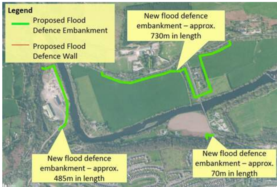
Figure 9: Defences at Inniscarra
