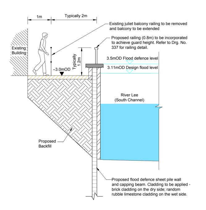
Section CIE-34 (Waterside Quay - Drg. No. LL\_227) Scale 1:50 @ A1, 1:100 @ A3
