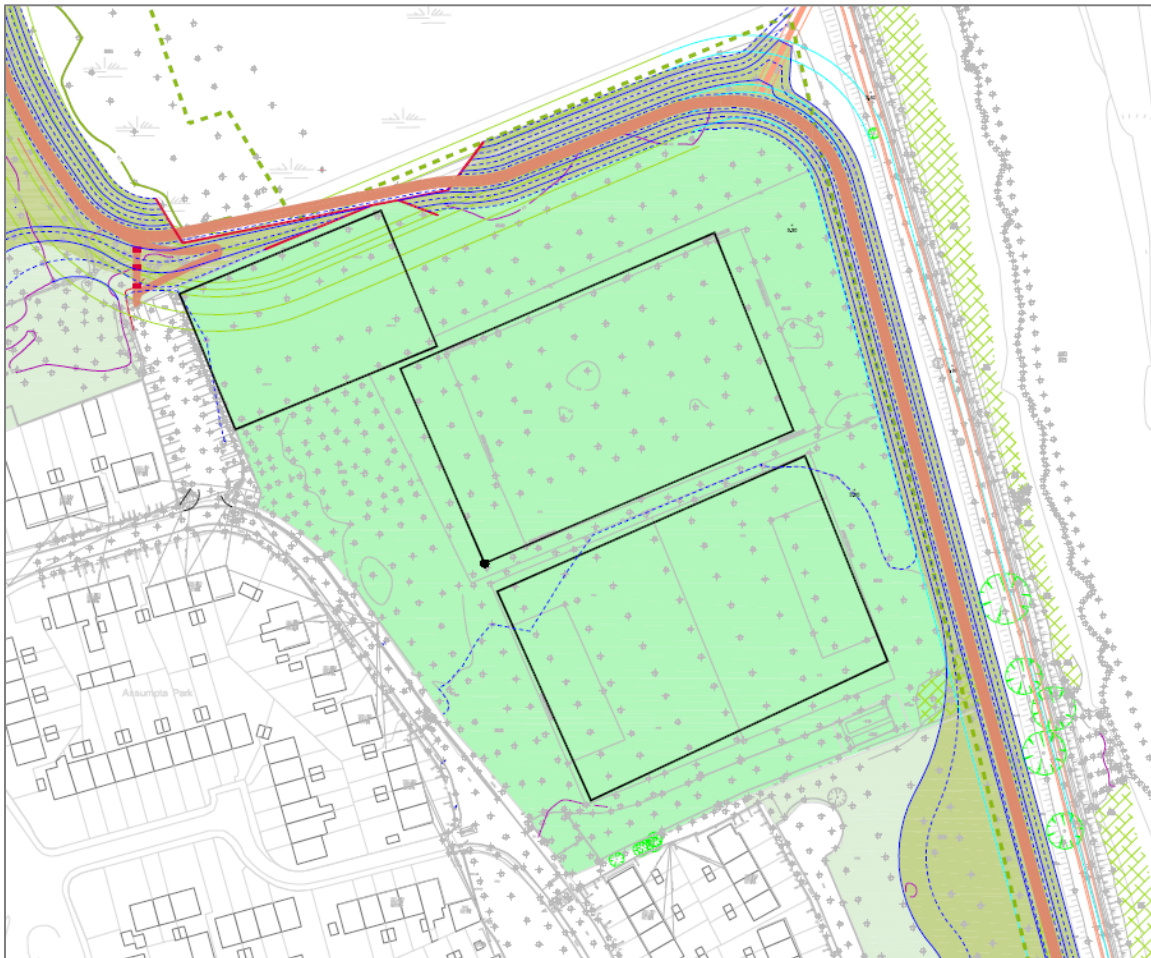
Figure 4-4 - Embankment and wall alignment at Star Rovers FC and Athlunkard Villa FC
