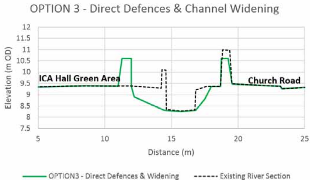
Figure 22: Option 3 - Typical channel cross section: ICA Bridge to Ravensdale Lower Bridge
