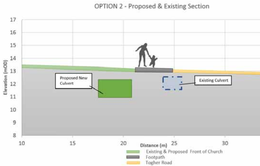
Figure 12: Option 2 – Indicative Cross Section at Church of the Way of the Cross (along Togher Road).
