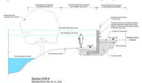
Figure 27: Section of Exhibited Defence Solution along Mardyke Arena
