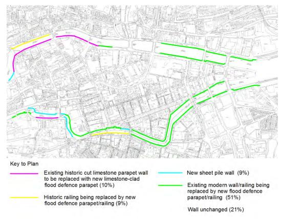
As can be seen, the majority of the existing parapet upstand walls and railings to be replaced are modern and will be replaced by an architecturally designed wall and railing combination which will take into consideration the existing aesthetics within the city.
