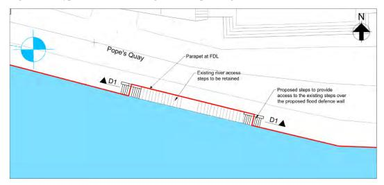
Figure 21: Typical Elevation #1 showing access steps being maintained
