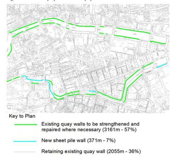
Figure 16: Extent of proposed works to quay walls
