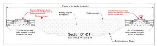
Figure 22: Typical Plan #2 showing access steps being maintained
