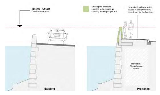
Figure 15: Typical Section of Proposed Quay Wall Works
