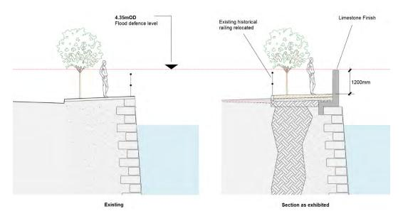
The solution as shown in Figure 45 & Figure 46 would limit the height of the parapet wall to no higher than normal minimum guarding height (1.2m). The proposed parapet wall was exhibited as a fair faced finished concrete. However, it was recognised that the actual finish would need further consideration, particularly in light of comments received from the public and other key stakeholders.
