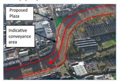
The proposed solution along Grenville Place involves the raising of existing road levels in order to achieve the required flood defence level, whilst maintaining a maximum parapet height of 1.2m. Figure 42 illustrates the difference between the existing and proposed scenarios. Figure 43 provides a photomontage of the proposed compared against the existing.
