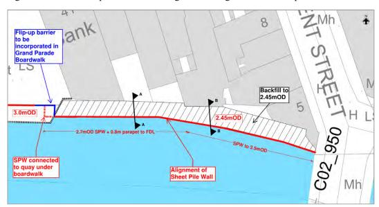
Figure 62: Plan of Proposed Defence Alignment along South Mall Properties
