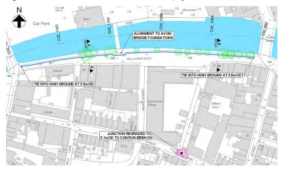
Figure 59: Plan of Alternative Solution for Sullivan's Quay
