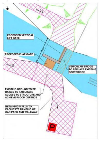
Figure 26: Plan of Proposed Flow Control Structure as exhibited
