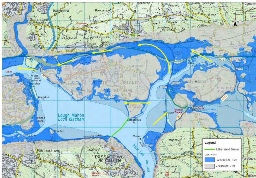
Figure 53: LiDAR Cut Section at 4.38m
