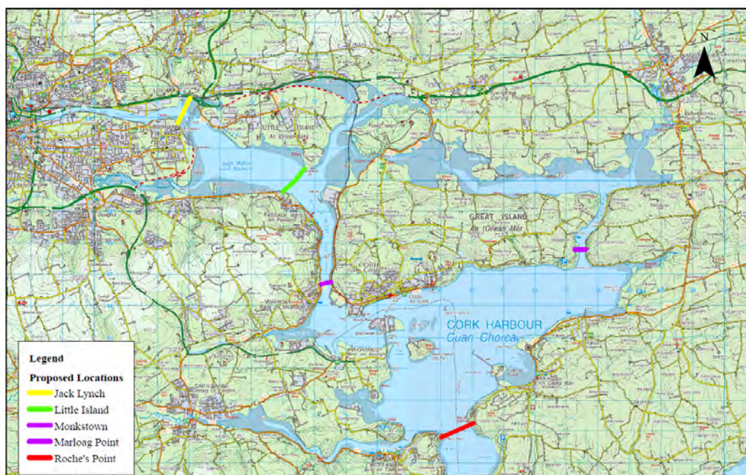
Figure 1: Potential Tidal Barrier Locations in Cork Harbour
