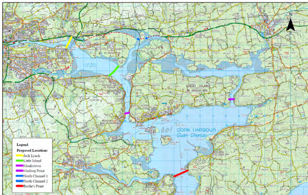
Figure 17: Cork Harbour – Potential Tidal Barrier Locations
