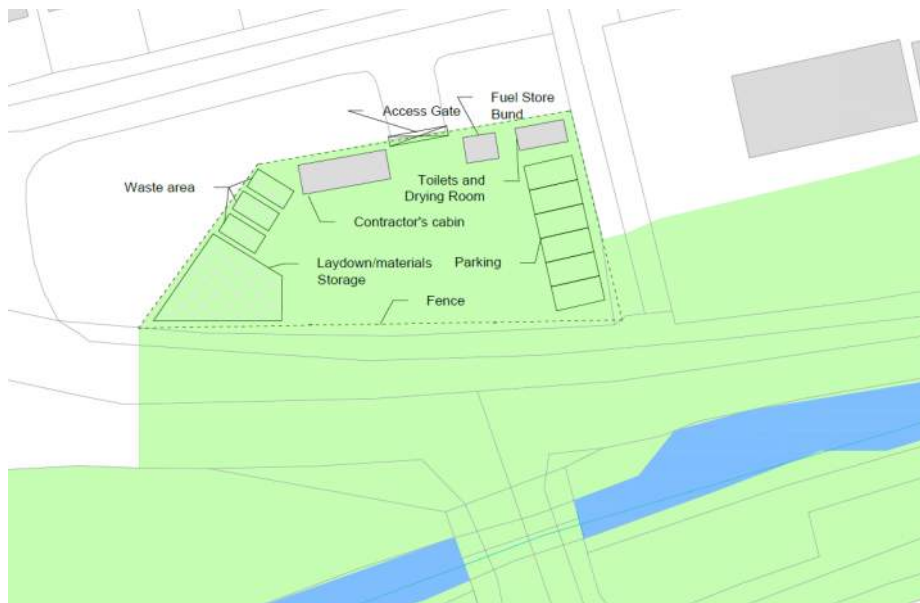
Figure 5.27 – Brooklodge Grove construction compound potential location
