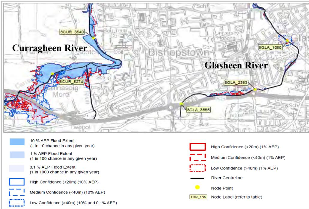
Figure 17: Extract from CFRAM flood maps showing upstream reach of Tramore River – Fluvial Flooding
