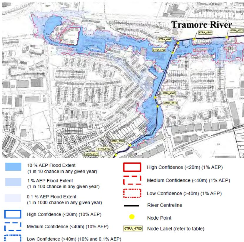
Figure 18: Extract from CFRAM flood maps showing Tramore River – Tidal Flooding
