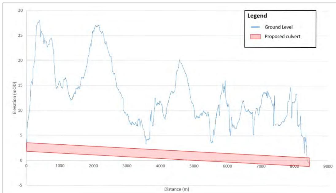
Figure 3 presents the proposed diversion overlain with LiDAR data to provide an indication of the changes in topography along the route. Figure 4 presents a long section profile plot of the proposed diversion route.
