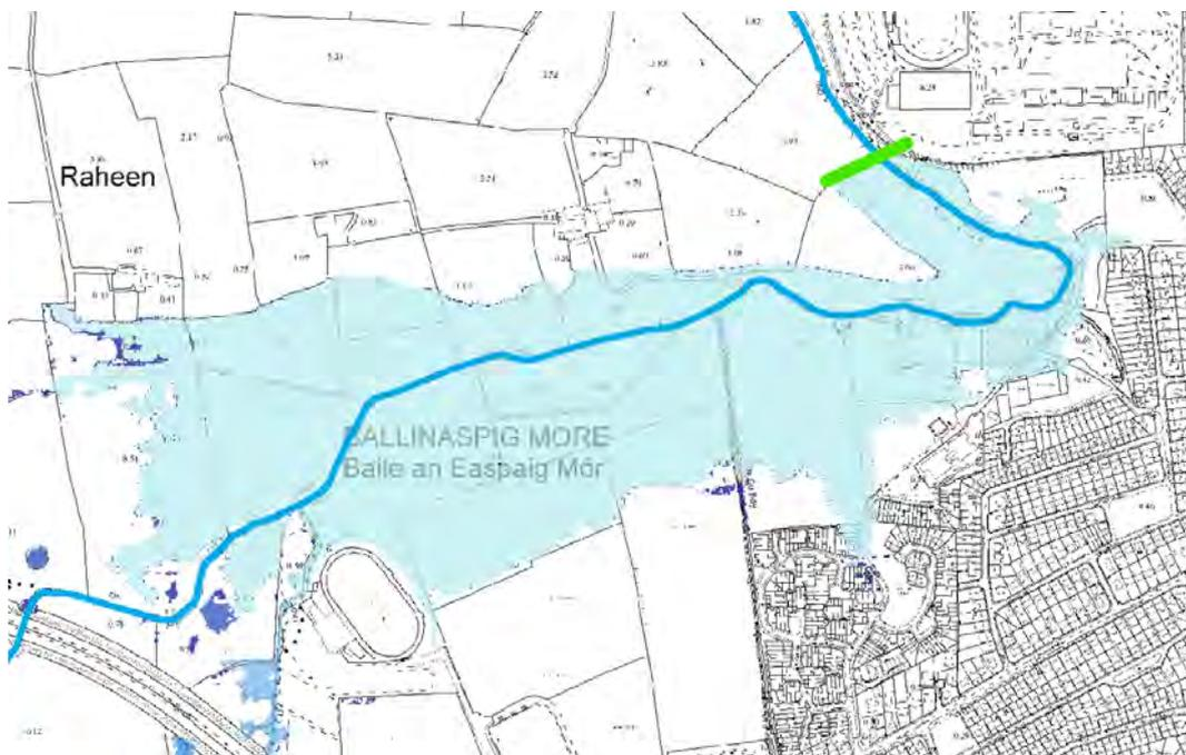
While the storage area is severely constrained by existing development in the area, there is the potential for approximately 550,000m<sup>3</sup> of storage to be created up to the 11mOD contour. This would involve the construction of a new dam (incorporating a flow control structure) with a maximum height of approximately 2m.
