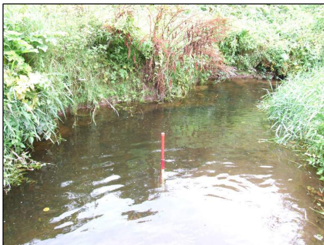
Plate 18: North-facing view of apex in river meander where the riverbed and west bank is subject to erosion (1m scale).
