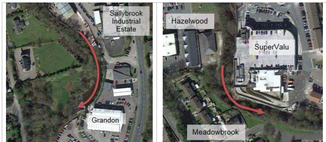
Figure 5-9: Bends at Grandons and Meadowbrook where superelevation is calculated
