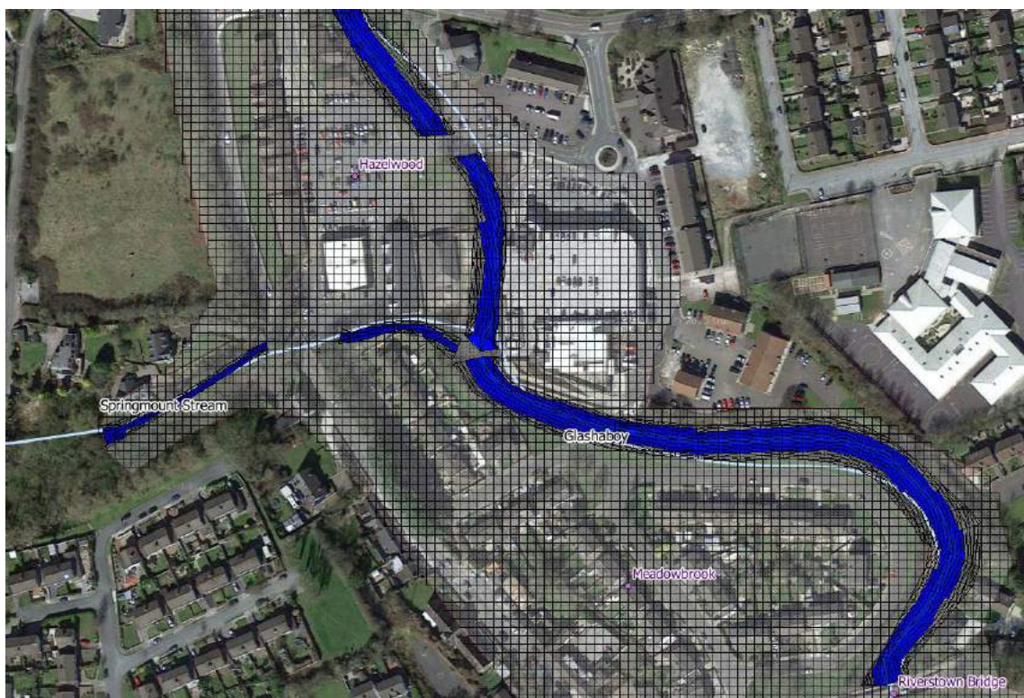
Figure 2-10 2D domain and grid through Hazelwood and Meadowbrook
