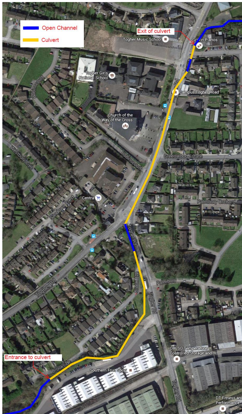
Figure 5: Schematic of the existing Togher Culvert and Open Channel
