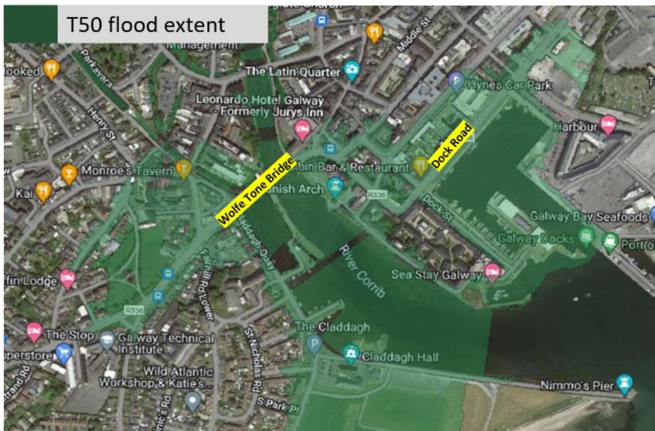
Figure 8.7.1 T50 tidal flood extents near the port area
