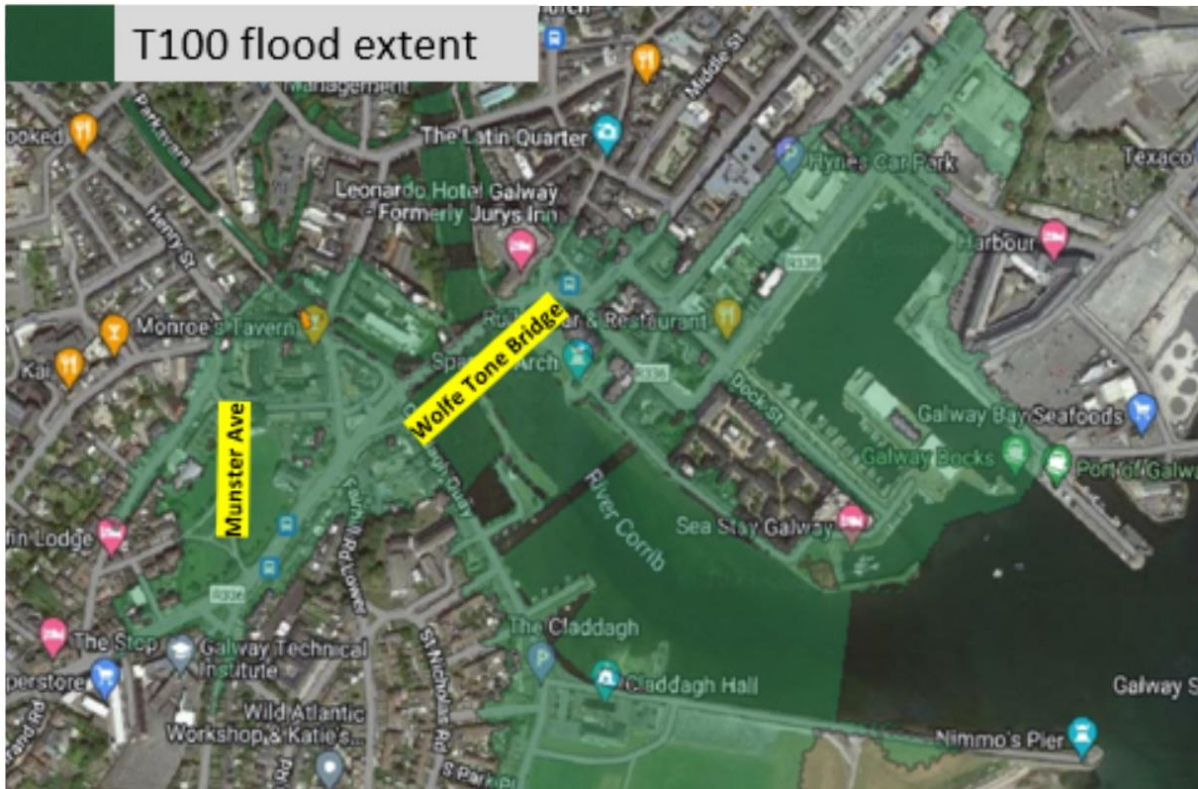
Figure 8.8.1 T100 tidal flood extents near the port area
