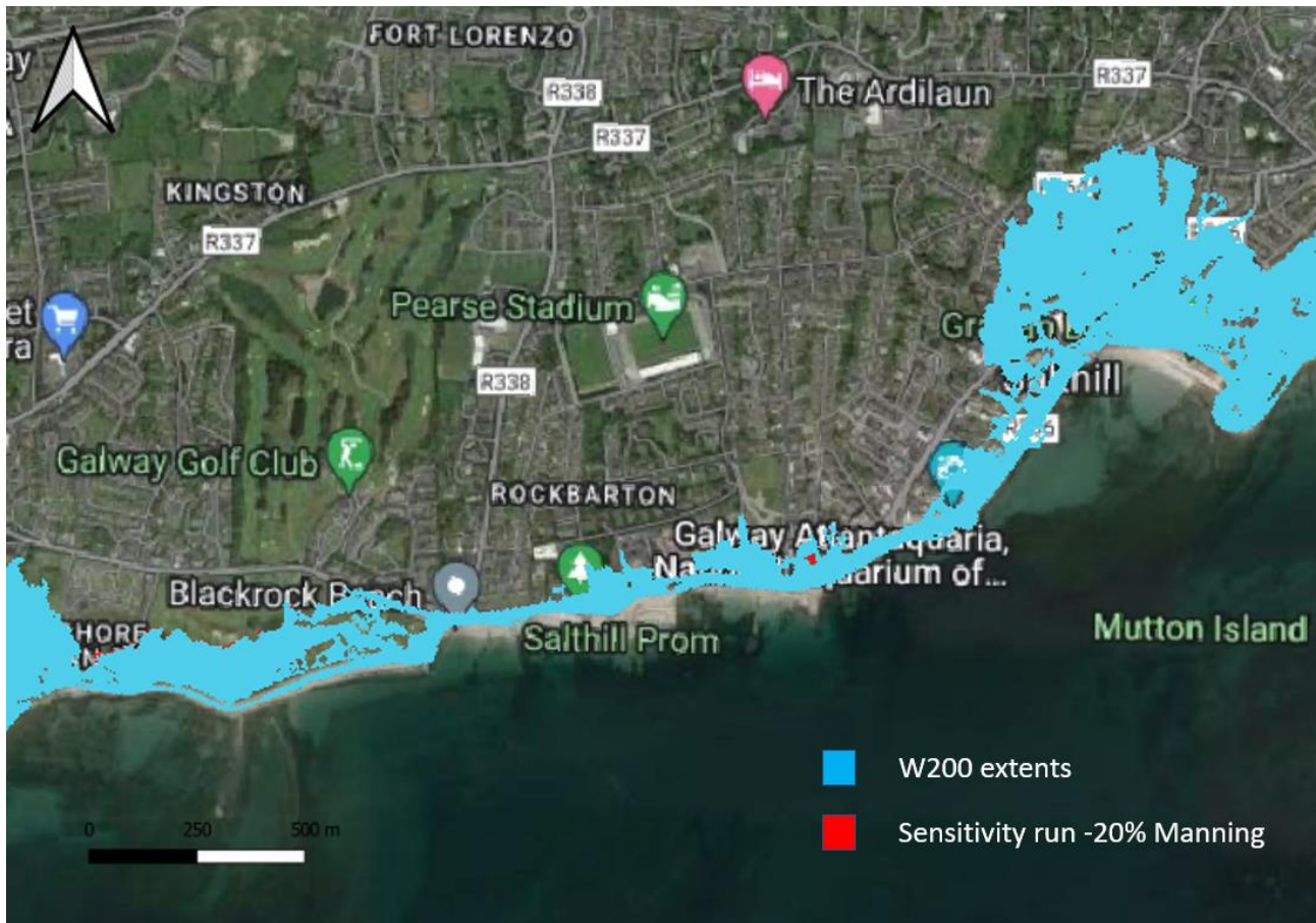
Figure 10.2.18 Comparison between W200 results and sensitivity run results with Manning's coefficient reduced by 20%.
