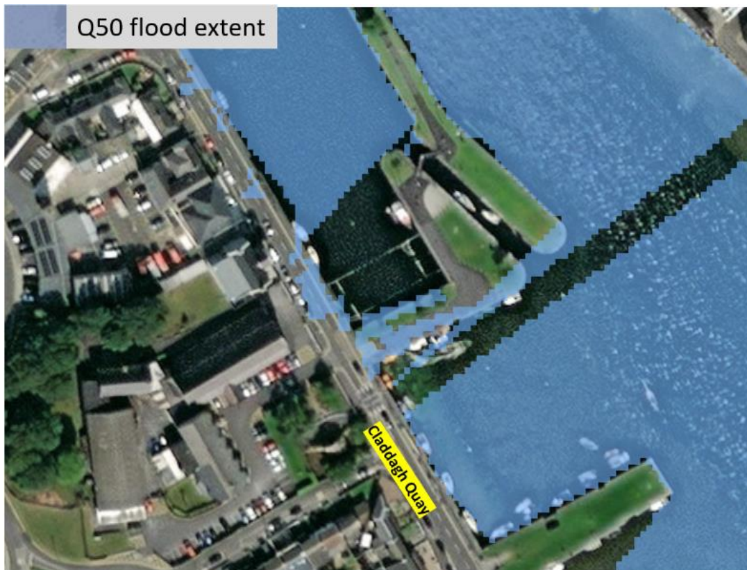
Figure 7.8.1 Q50 fluvial flood extents near the Dyke Road embankment
