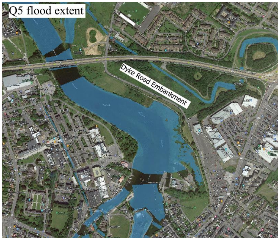
Figure 7.5.1 Q5 fluvial flood extents around the Dyke Road embankment
