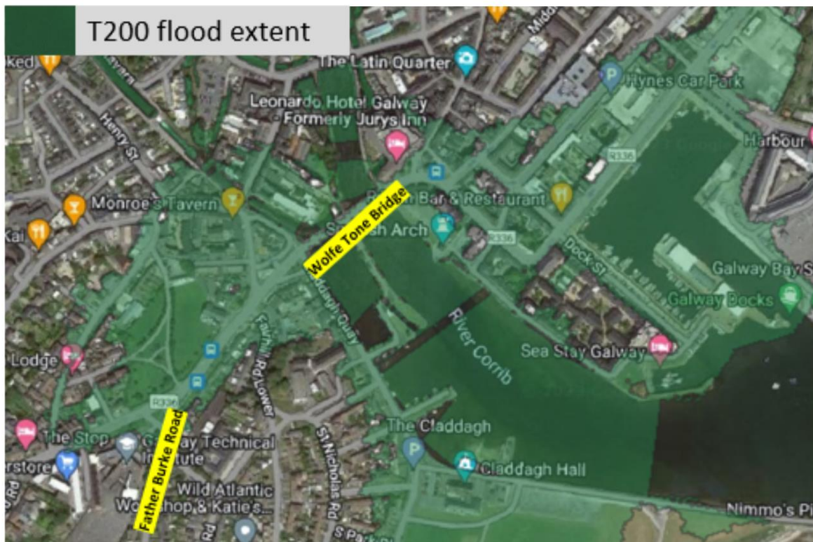
Figure 8.9.1 T200 tidal flood extents near the port area
