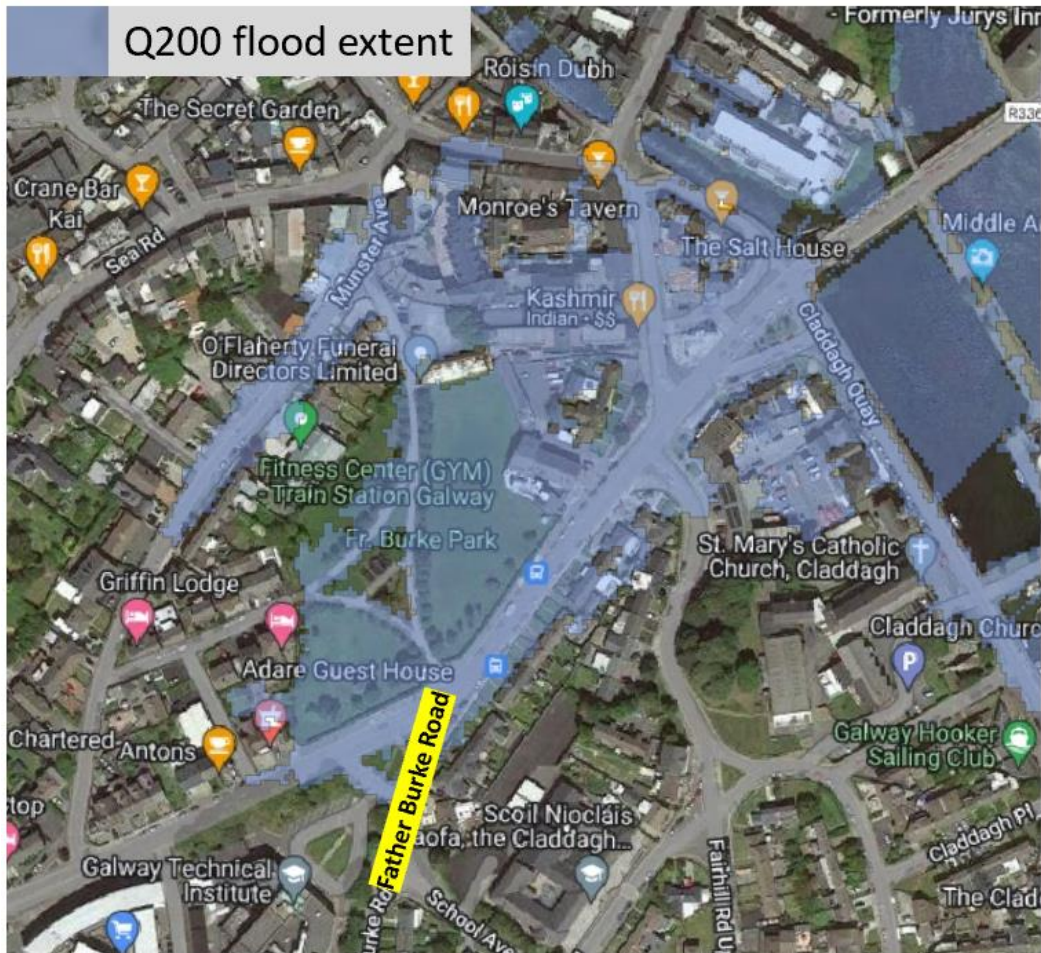
Figure 7.10.1 Q200 fluvial flood extents near Claddagh Quay
