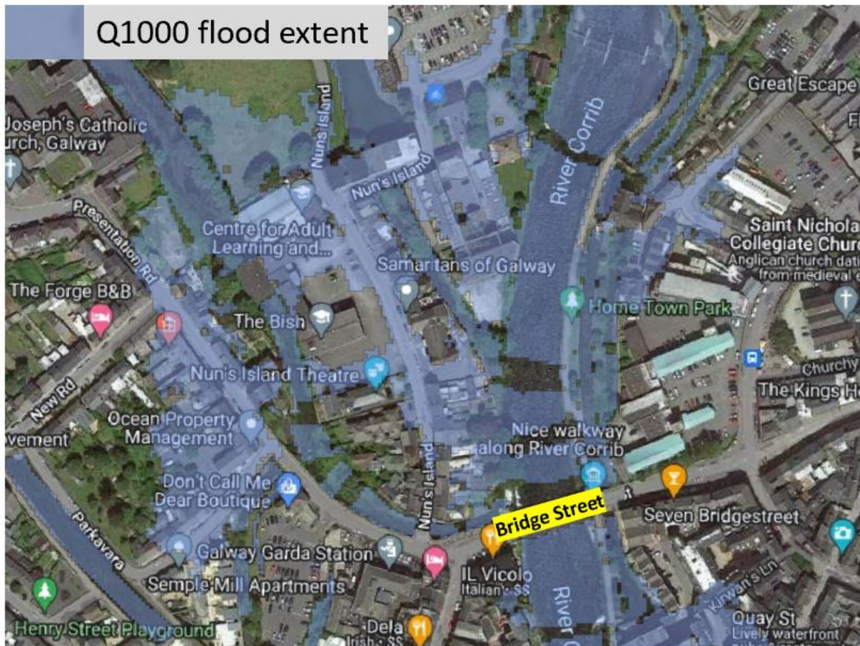
Figure 7.11.2 Q1000 fluvial flood extents near Bridge street
