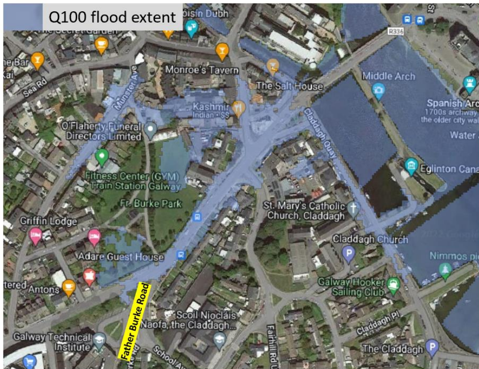
Figure 7.9.1 Q100 fluvial flood extents near Claddagh Quay
