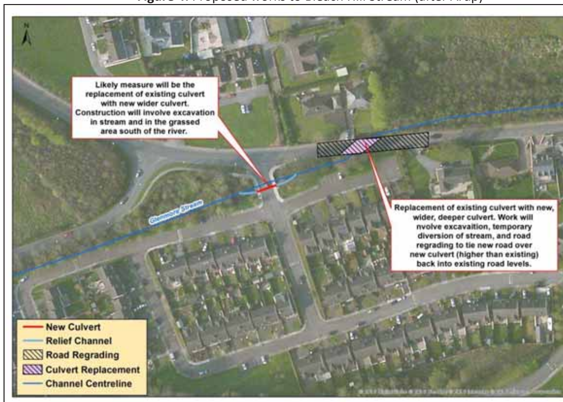
Figure 5: Proposed works to Glenmore Stream at Copper Valley Vue and culvert under Brooklodge Grove Road (after Arup)
