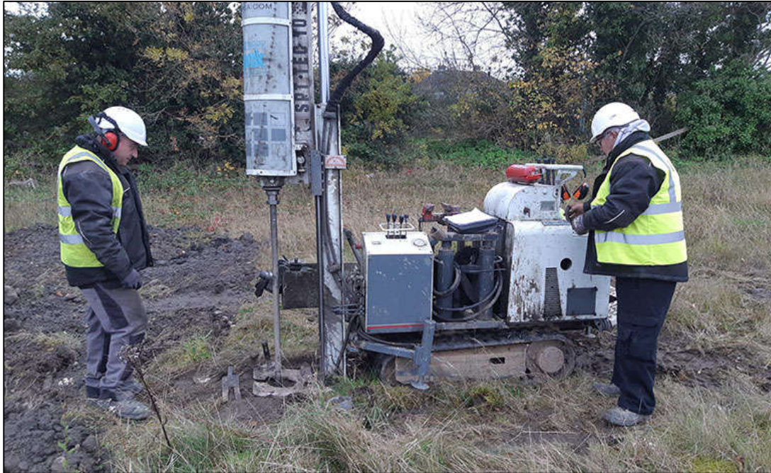
Figure 5.4. Photo of typical dynamic probe operation.
