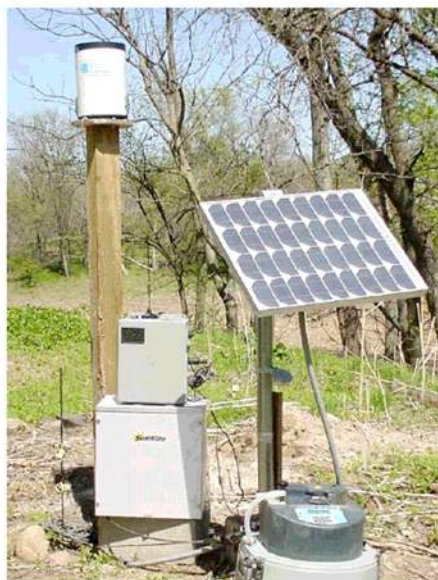
A 674 rain gauge connected to an Isco 6712 or Avalanche sampler is ideal for collecting rainfall data as well as runoff-triggered samples at remote monitoring sites.
