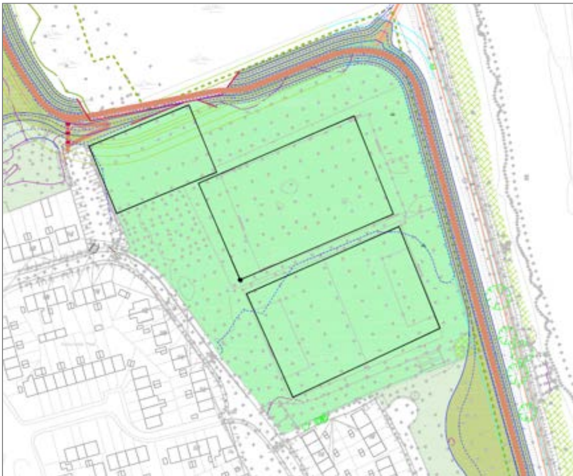
Figure 12-3 - Embankment and wall alignment at Star Rovers FC and Athlunkard Villa FC
