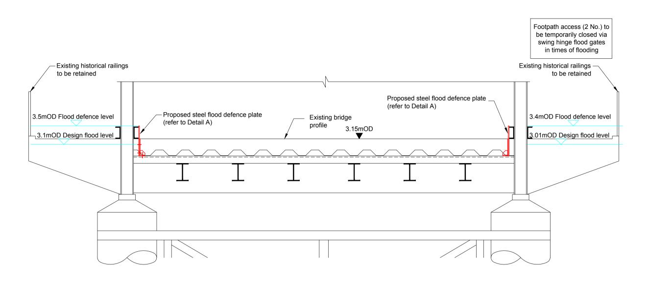
Section SSC-4 (Clontarf Bridge - Drg. No. LL\_224) Scale 1:50 @ A1, 1:100 @ A3
