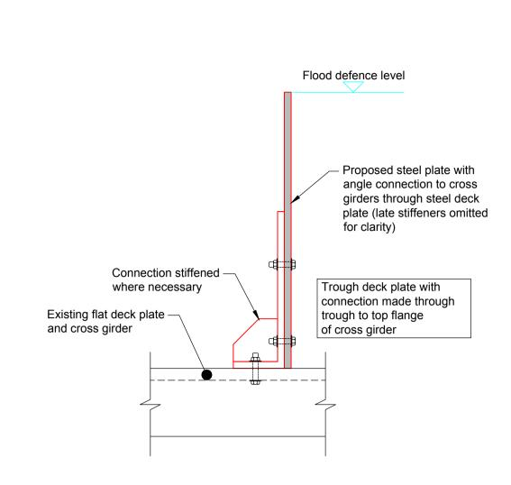
Detail SSC-A Scale 1:10 @ A1, 1:20 @ A3
