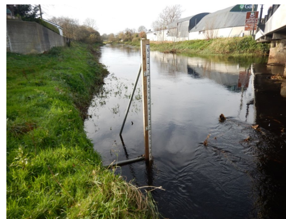
Figure 3 - Gauging station. Photo taken as part of topographic survey.
