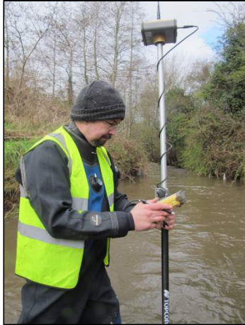
Plate 1: Working shot of DGPS being used to record a river profile, River Area 3.
