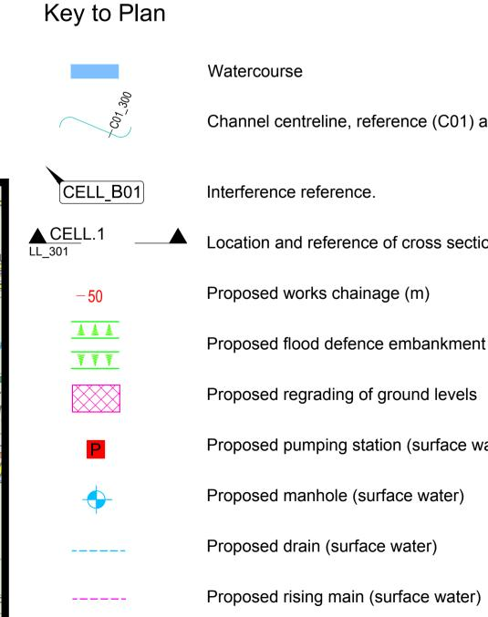
Channel centreline, reference (C01) and chainage (300m) Interference reference. Location and reference of cross section Proposed works chainage (m) Proposed flood defence embankment Proposed regrading of ground levels Proposed pumping station (surface water) Proposed manhole (surface water) Proposed drain (surface water)
